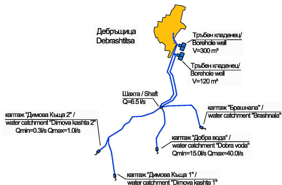
Figure: Layout of the water supply system Debrashtitsa
