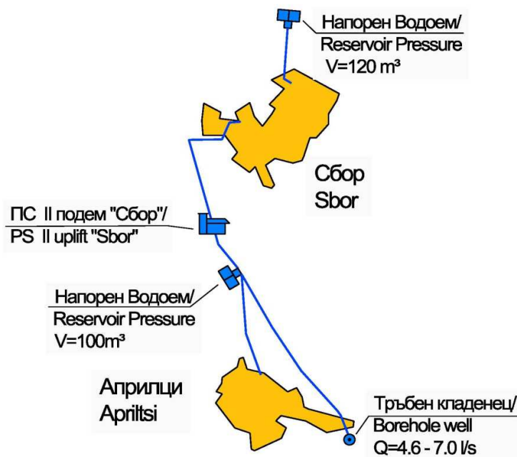
Figure: Layout of water supply system Apriltsi – Sbor
