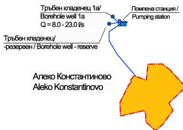
Figure 3-7 Layout of water supply system Aleko Konstantinovo
